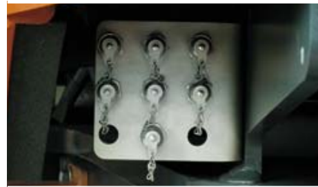
Central Remote Hydraulic Check Port The centralized remote hydraulic check ports allow main, steering, brake charge, pilot, load-sensing signal and transmission clutch pressures to be checked at a convenient central location.
