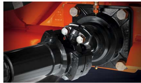
Propeller Shaft A protective cover has been installed to protect the oil seal from dust, foreign objects and premature wear.
