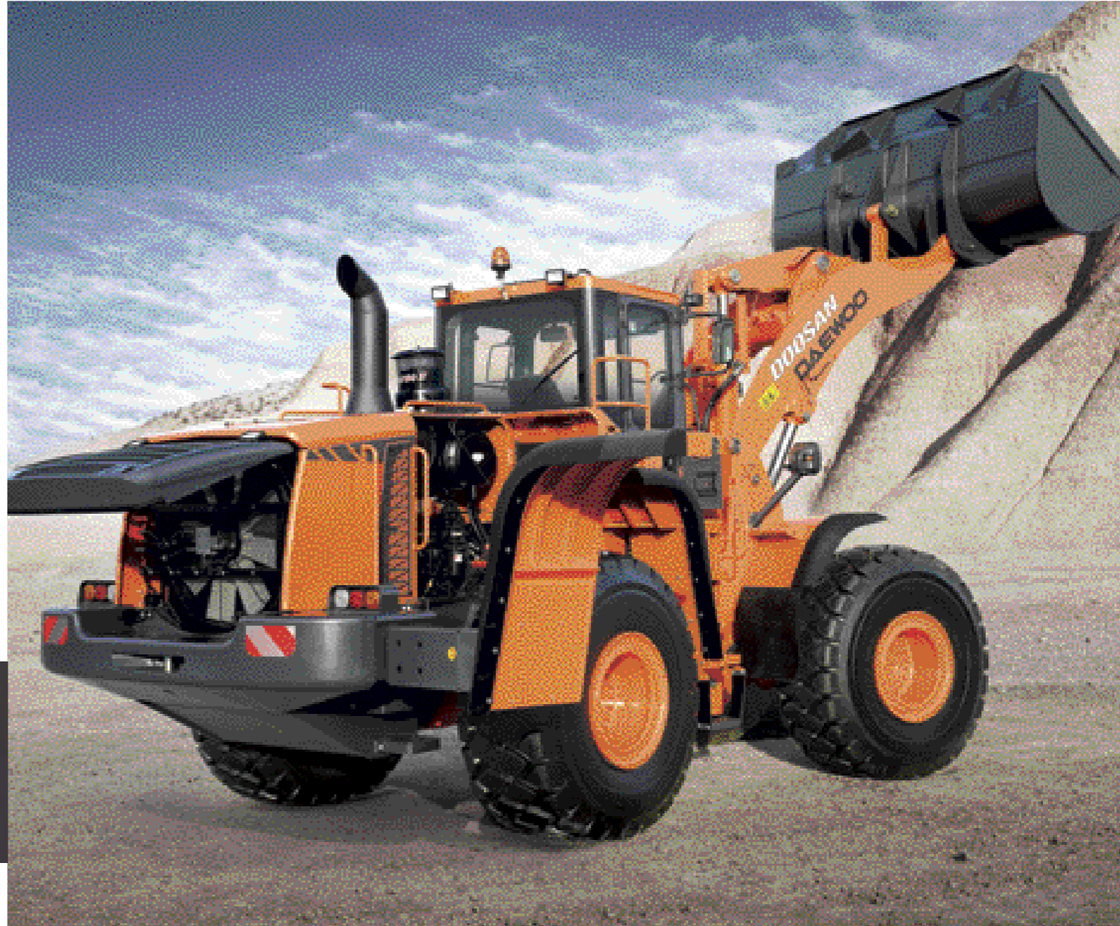
Hydraulically operated reverse fan With electronic control of the variable speed on-demand fan, temperature levels of the engine coolant, transmission oil are constantly monitored. Controlled fan speed improves fuel efficiency, lowers noise levels and reduces radiator plugging. The hydraulic fan can be switched to reverse operation from the cabin for quickly clean out the cooling system.
