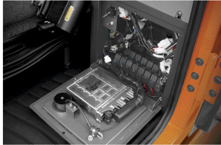
Transmission & Engine Diagnosis The transmission and engine can be diagnosed using a laptop computer to interface with the diagnostic system.
