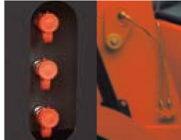
Remote Greasing Lubrication Ports The front pins can be lubricated from the outside of the machine without crawling under the machine or in awkward positions through the lubrication ports.
