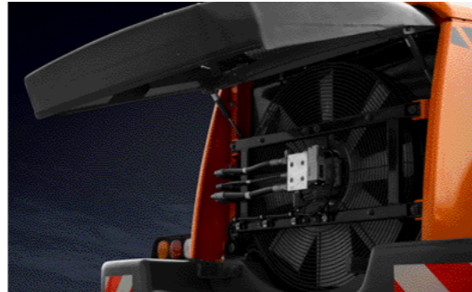
Hydraulically operated reverse fan With electronic control of the variable speed on-demand fan, temperature levels of the engine coolant, transmission oil are constantly monitored. Controlled fan speed improves fuel efficiency, lowers noise levels and reduces radiator plugging. The hydraulic fan can be switched to reverse operation from the cabin for quickly clean out the cooling system.
