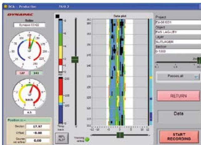
*The pass-count and asphalt temperature are presented in real-time on the operator screen - providing vital information for a successful compaction job.*
